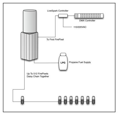
FirePixels were designed for ultimate ease of use, portability, control, and safety. Each FirePixel responds 30 times per second and offers 256 selectable heights, to create smooth animations with low latency. The LiveSpark Controller works seamlessly with the lighting programs you are
